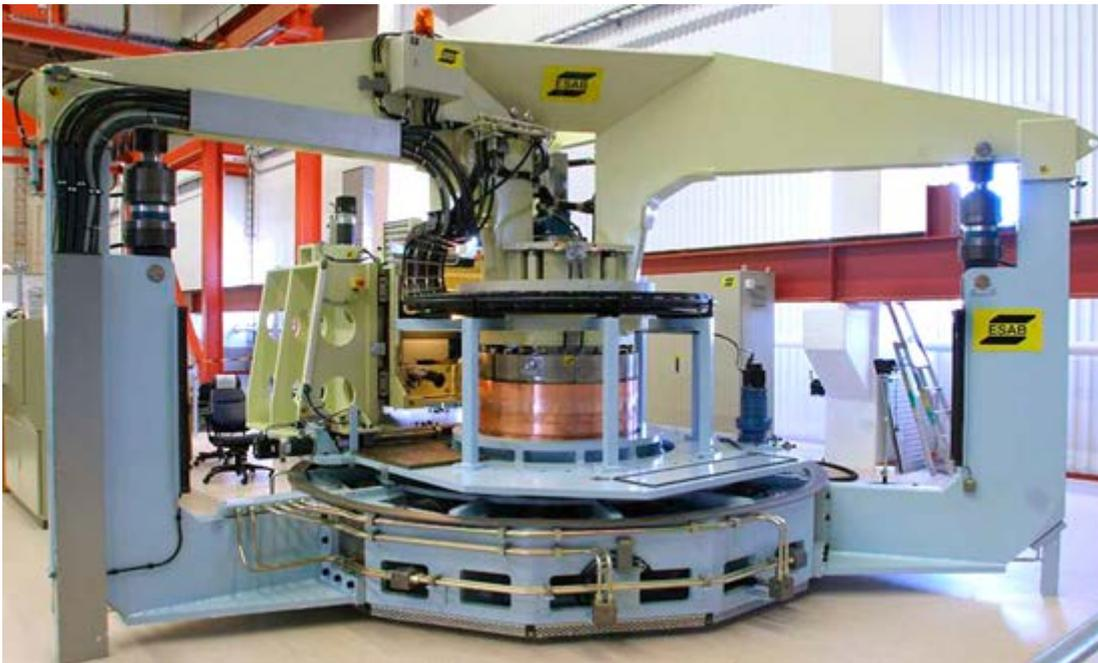
**Figure 1-2.** Purpose-built FSW machine for copper canister welding, before the argon gas shield was installed.
